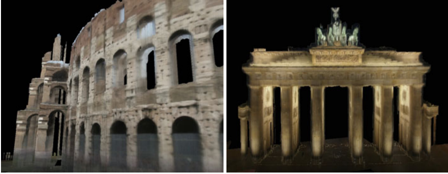
Fig. 1. Example models of our method from Rome (left) and Berlin (right) computed in less than 24 hours from automatically registered subsets of photo collections of 2.9 million and 2.8 million images respectively
